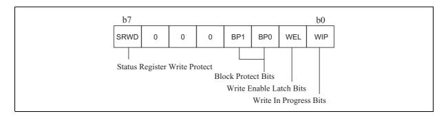
WIP bit: The Write In Progress (WIP) bit indicates whether the memory is busy with a Write or Write Status Register cycle.
